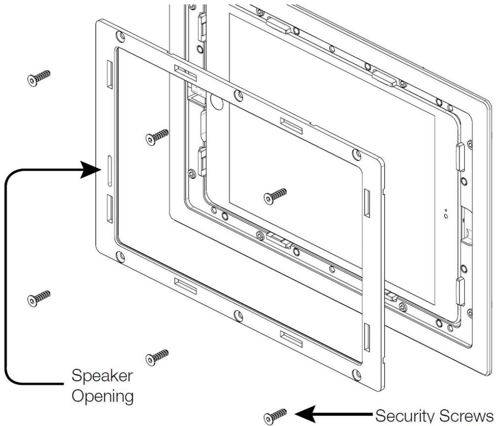
Place the magnetic retaining ring over the tablet, making sure that the opening for the speaker is oriented correctly.
