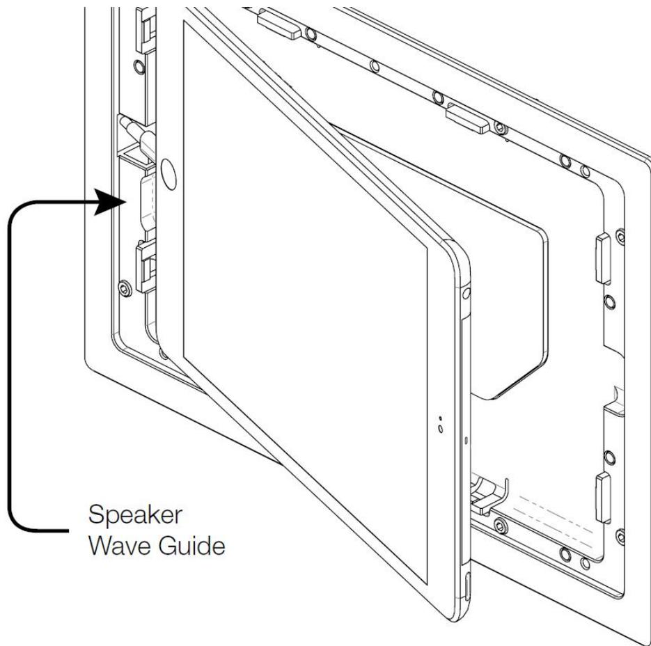
Attach the charging cable to the tablet and carefully position the charging connector through the opening of the bracket frame.
