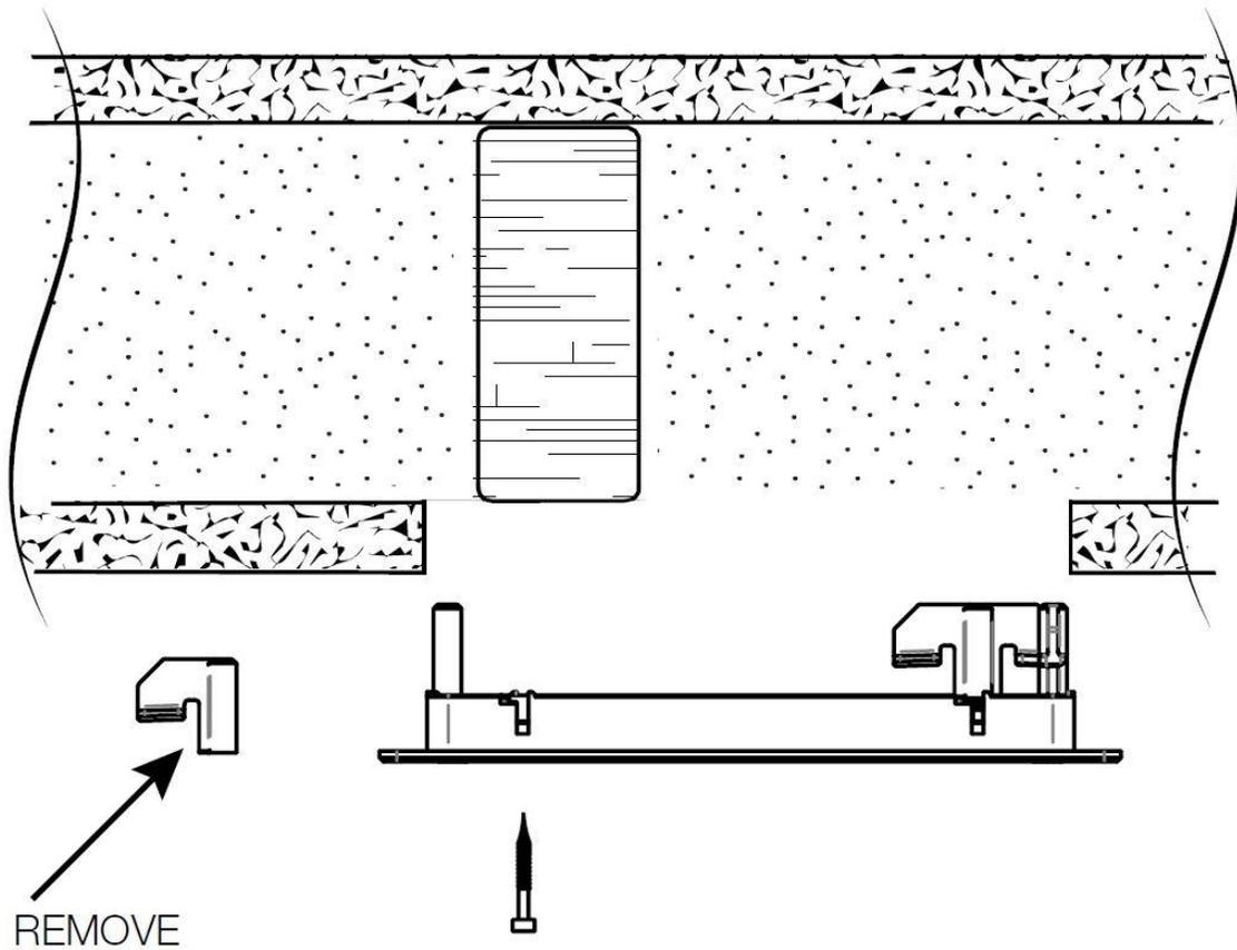
If the opening in the drywall is obstructed by a wooden stud or other obstruction, it may be necessary to remove one or more of the dog-ears.
