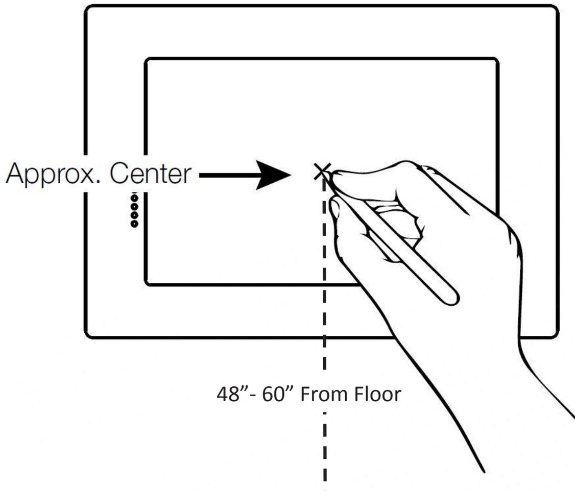
The FitnessOnDemand™ touch screen kiosk is designed to be mounted horizontally in locations where 1/2" or 5/8" drywall has been installed. Because of the shallow depth of the in-wall bracket, it is not necessary to limit placement only to areas between studs.
