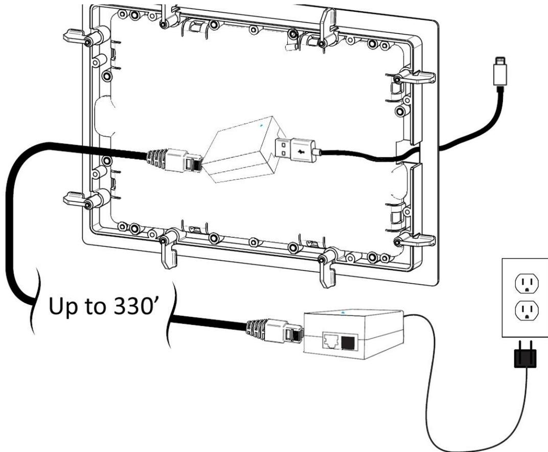
The included PoE to USB receiver and PoE Injector work together to provide 2.1A (10W) charging to your FitnessOnDemand™ touch screen tablet through up to 330' of Cat5 or Cat6 Ethernet cable.
