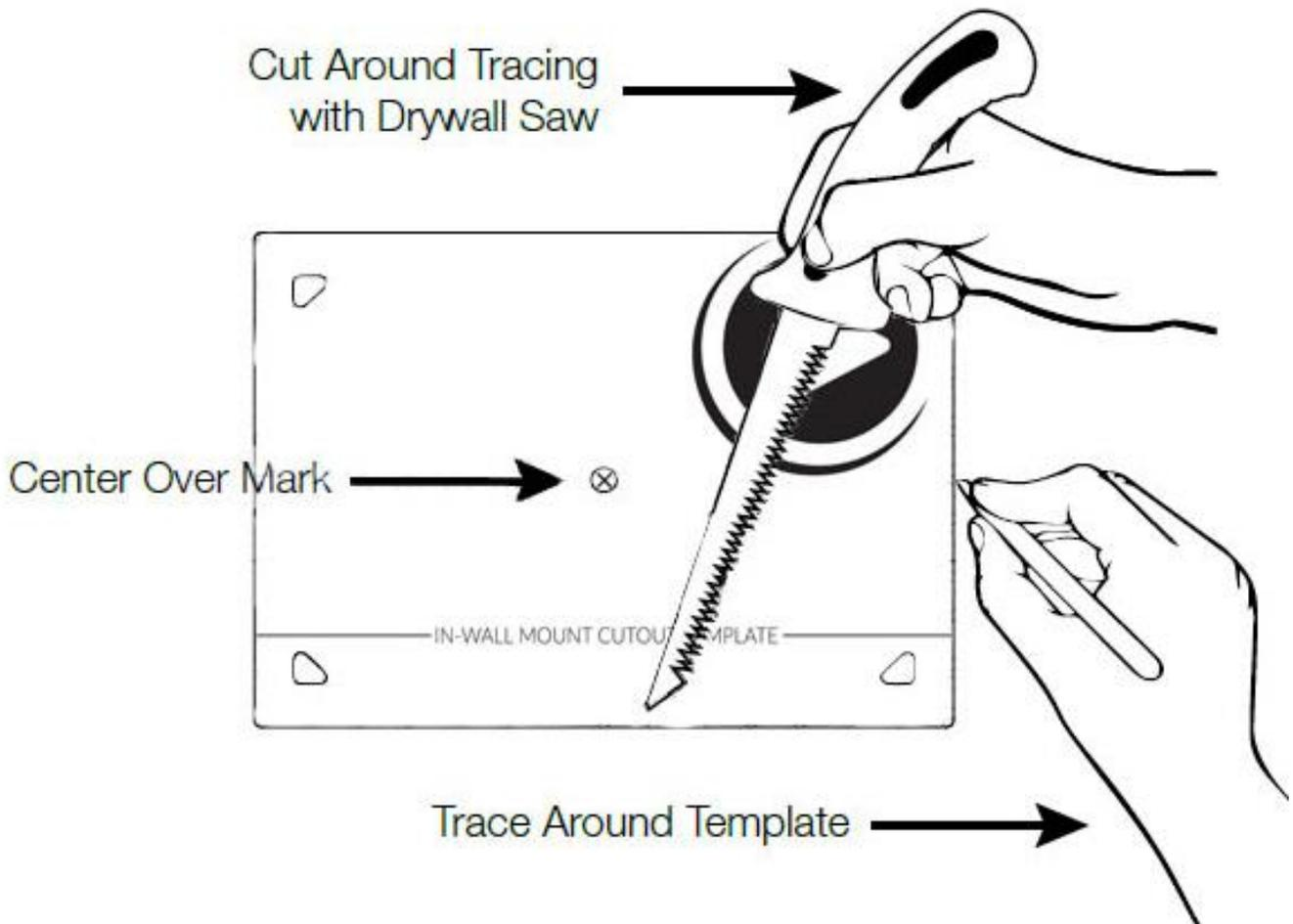
Using a level, center and place the included cutout template over the center point mark. Trace and then cut the opening using an electric rotary tool or drywall saw, taking care not to damage any wiring, plumbing or ductwork inside the wall.
