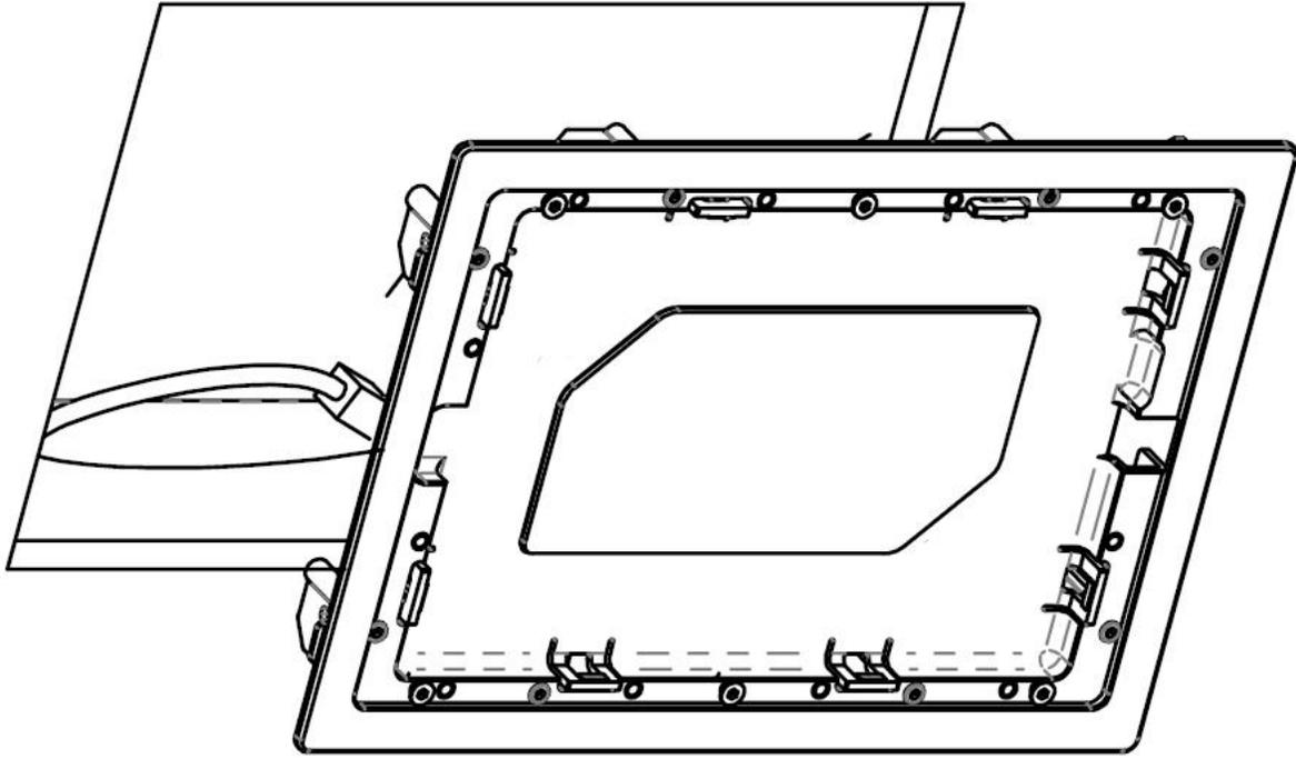
Remove the steel faceplate as well as the plastic retaining ring from the in-wall bracket and set them aside.
